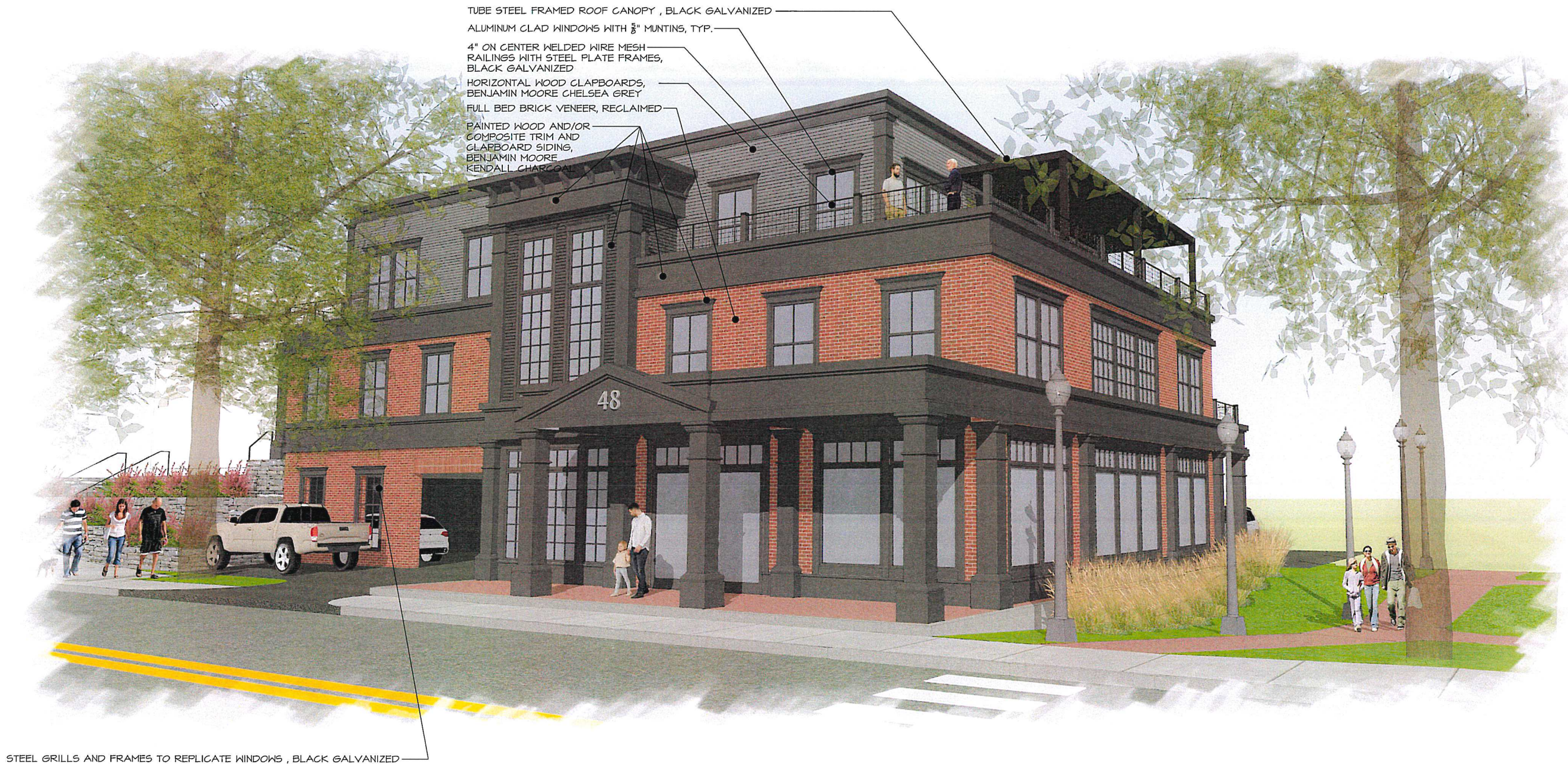
STEEL GRILLS AND FRAMES TO REPLICATE WINDOWS, BLACK GALVANIZED PROPOSED EXTERIOR RENDERING FROM SOUTHEAST
