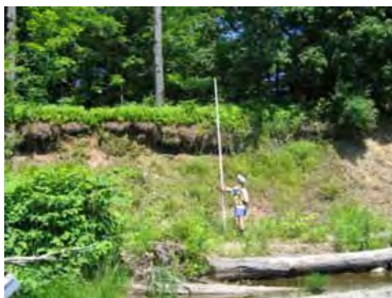
Figure 7.38. Mass failure 20 feet high along eastern bank in Reach T4.01
