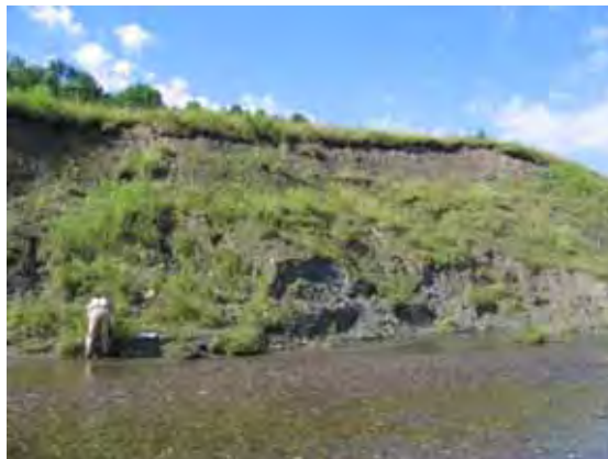
Figure 7.63. Mass failure acting as a major sediment source in Moss Glen Brook in T8.01-B
