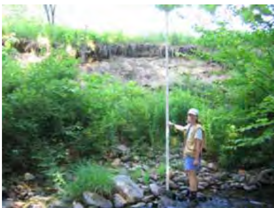
Figure 7.37. Mass failure 12 feet high along western bank in Reach T4.01
